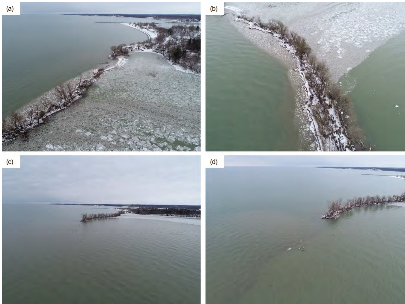
Figure 4-9. Recent drone images, collected February 11, 2020, showing current and ongoing deterioration of the eastern (a,b) and western (c,d) reaches of the Blind Sodus Bay barrier bar.
