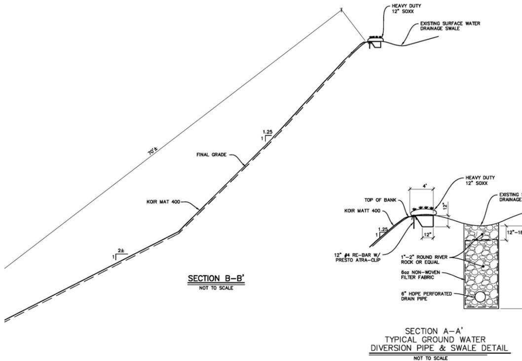
**Figure 4-4** Regraded Slope
