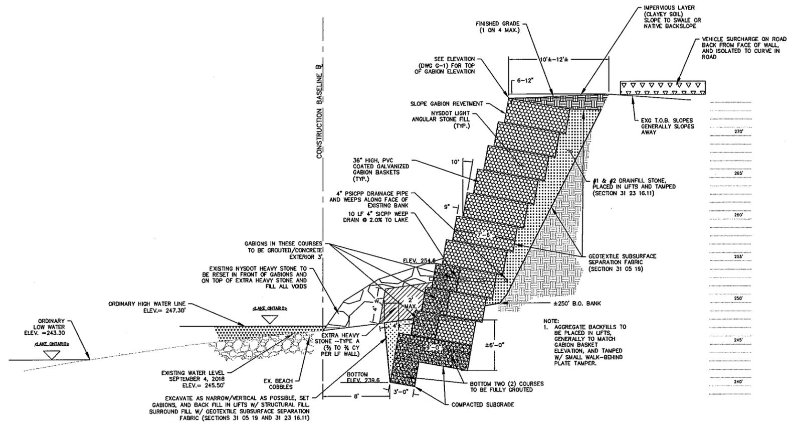
**TYPICAL CROSS SECTION - GABION INSTALLATION**
