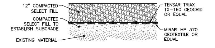
Figure 4-6 Typical Section Roadway Repairs to elevation 251 ft
