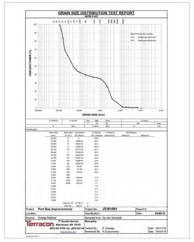
Figure 2.1-51 Gradation Curve for Sample from 2018 Channel Dredge Material
