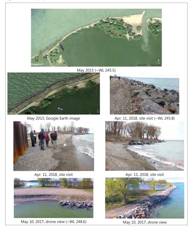
Figure 2.1-20 Riprap Protection of the West Barrier Bar; 1,700 ft of Rock Revetment
