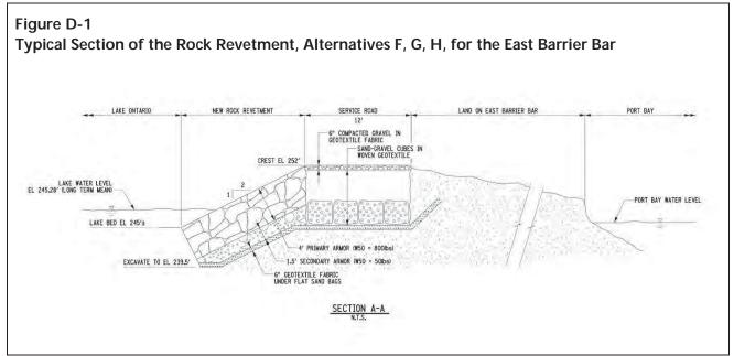
*Note:* Where the bar EL > 252 ft, the cubes may not be needed, and the road is built on natural land in cut.
