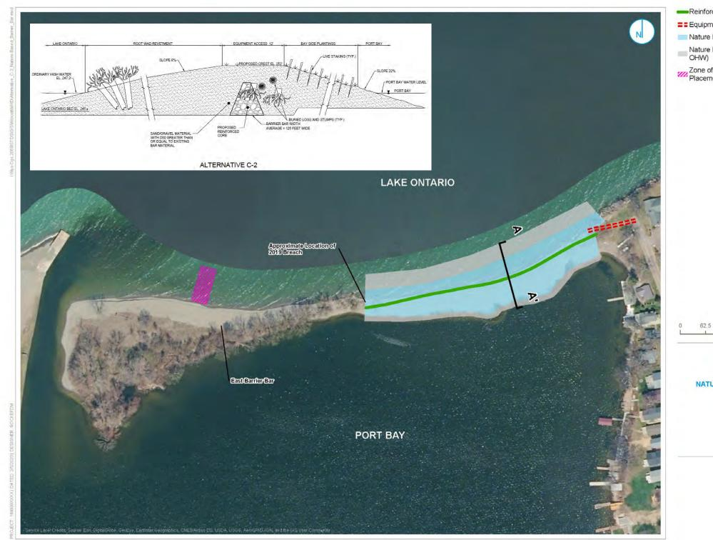
Figure 4-1 Alternative C-2: Nature-Based Barrier Bar with Reinforced Core
