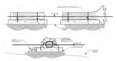
SINGLE LOG-BASED BREAKWATER - CONCRETE BALLAST
