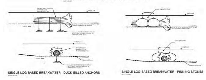
Figure 4-3 Typical Woody Breakwater Structures, Depicting Concrete, Duck-Billed Anchors, or Pinning Stones as Ballast
