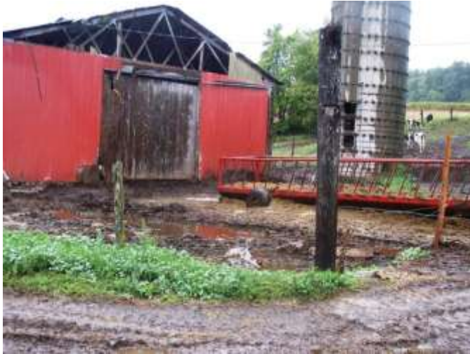
Barnyard area in need of runoff structures, heavy use stabilization, and manure management structures.
