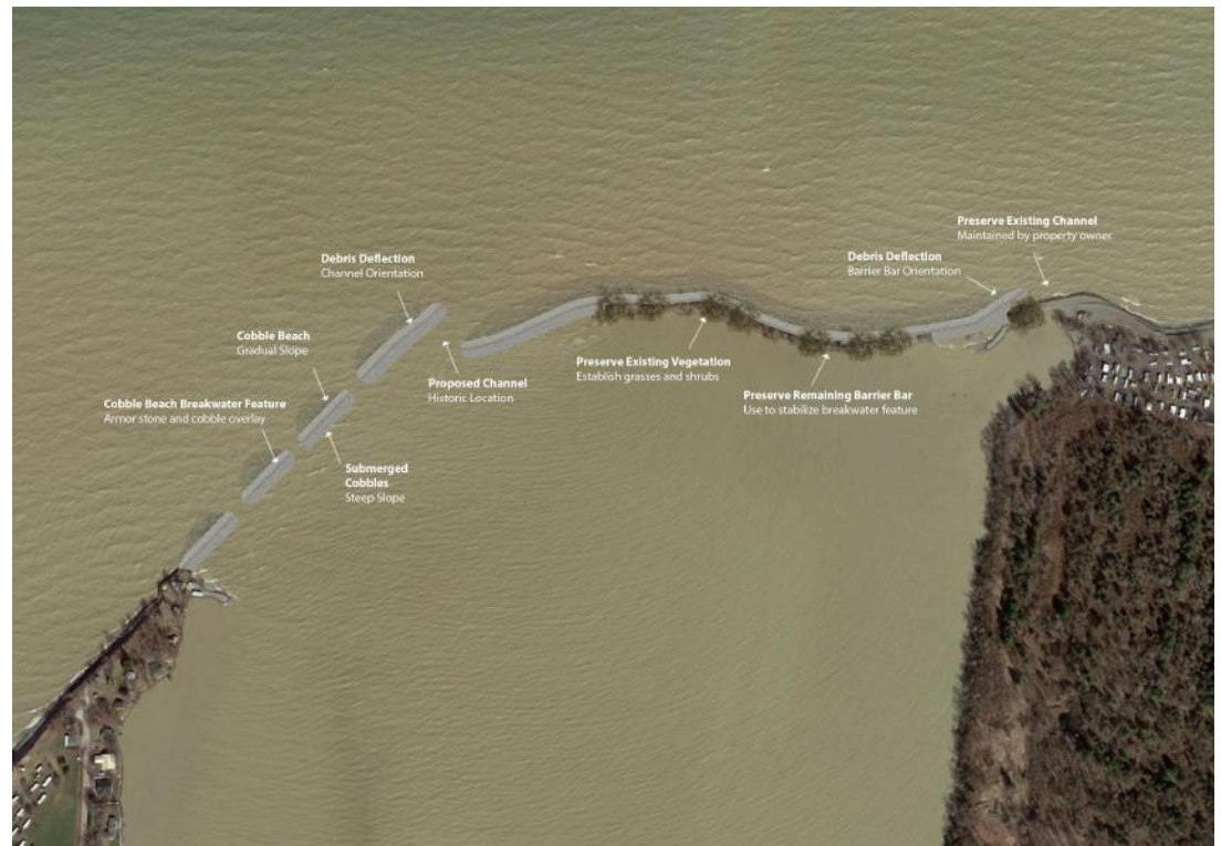
Preferred Alternative: Barrier Bar Breakwaters, Re-Establishment, and Enhancement with Naturalized Channel and Debris Deflection in Historical Location, and Sediment Deflection in Current Channel Location
