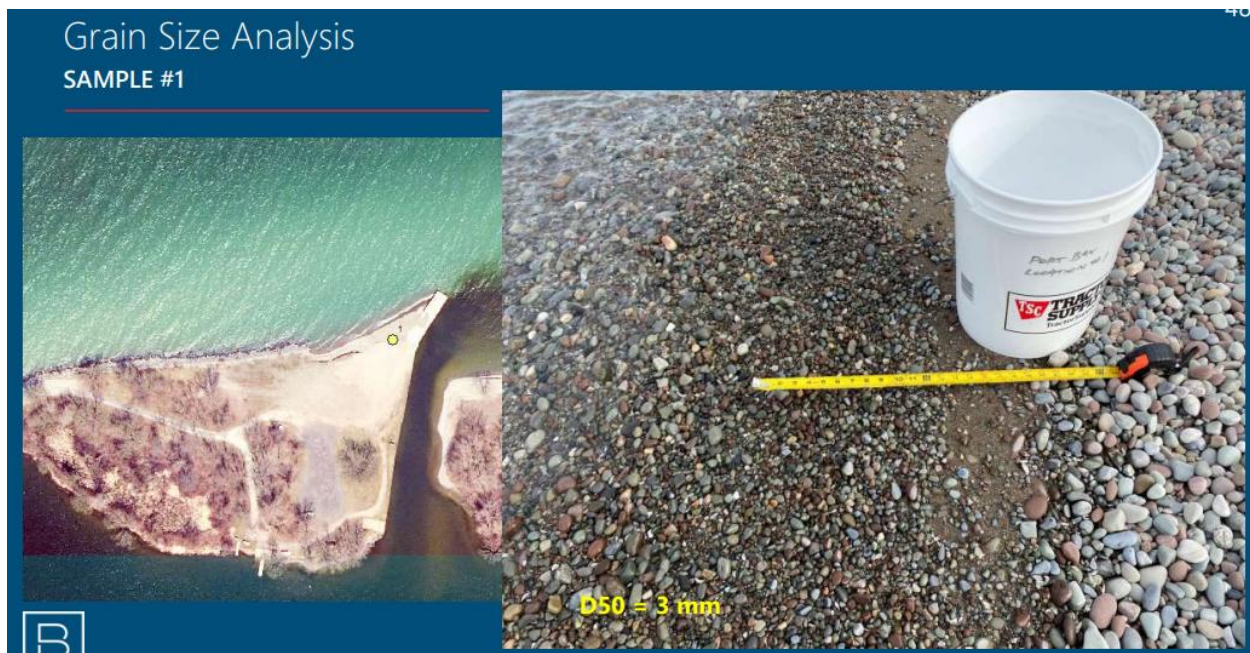
Figure 28 – Sediment sample location #1 ( D_{50} = 3\text{mm} )
