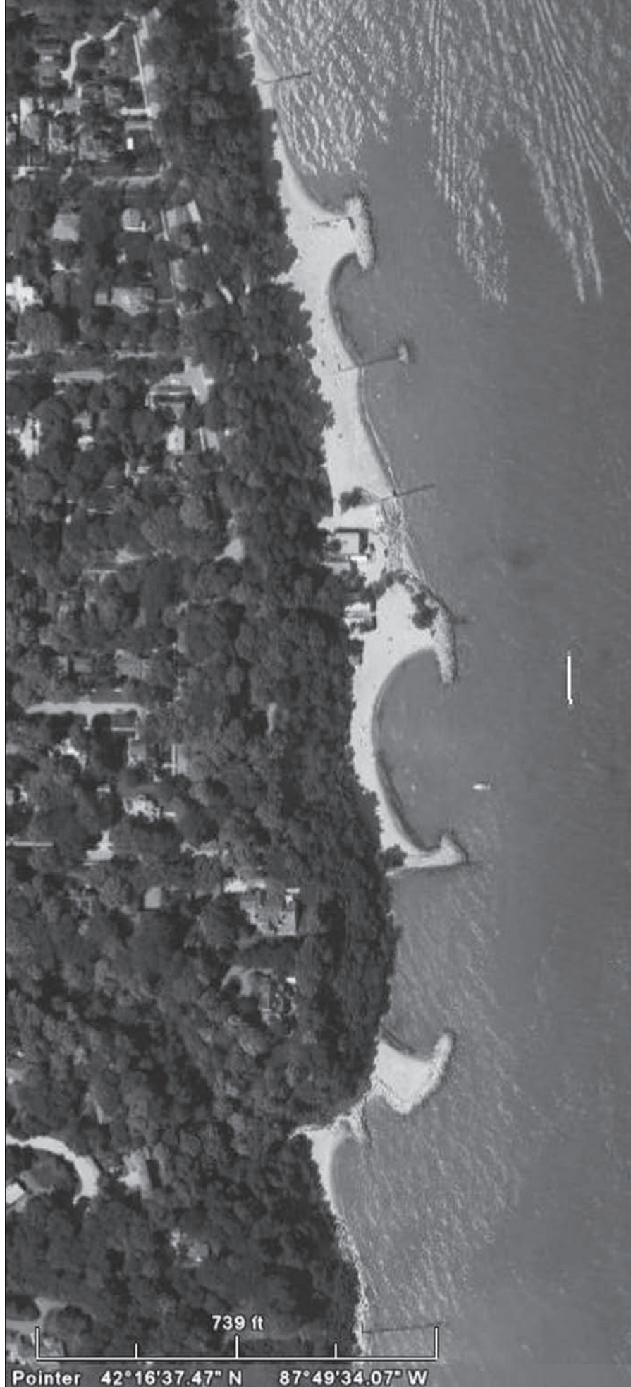
Figure 9. Sunrise Park Beach, Lake Bluff, Illinois, Lake Michigan. South Beach (project beach) opposite 100-ft scale bar, with spur breakwater on the north side of the beach cell and armored headland on south side of cell. North Beach (control beach) with new headland breakwaters at top of photo. Google air photo, 11 October 2007.
