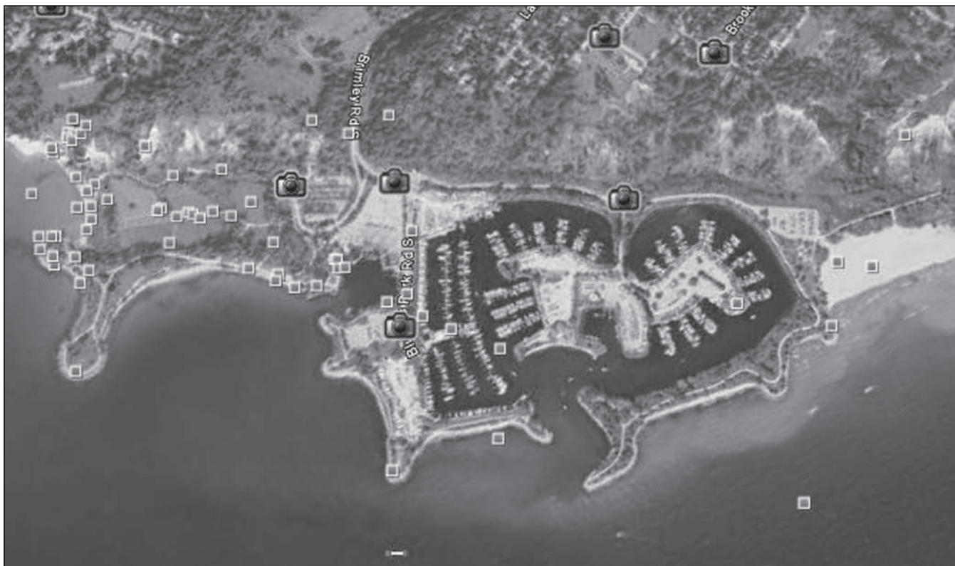
Figure 5. Built on reclaimed land in Lake Ontario east of Toronto, Bluffer's Park first opened in 1975 and was expanded to its current size in the early 1980s. The park is home to four sailing clubs. Note 100-ft scale bar and armored headland on left (Google air photo 2009).
