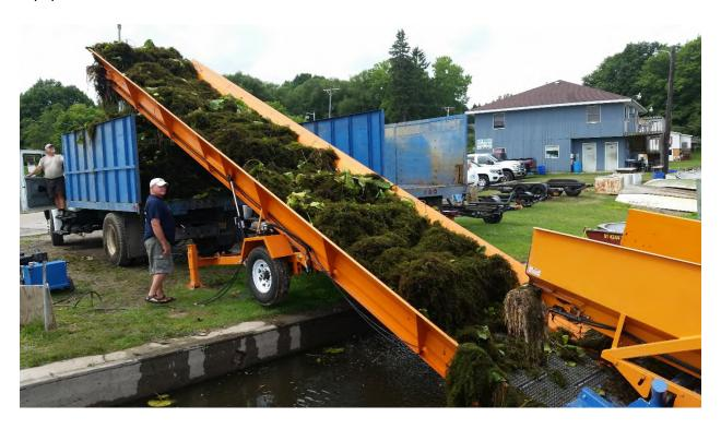
The pattern of operation for harvesting aquatic plants varies per situations, conditions, and locations. The most common pattern is to harvest from docks-end outward to a point in which the 'weeds' become less dense and mechanical harvesting efficiency lessens. The annual goal of the program is to capture and remove 500 harvester loads of nuisance aquatic plant material from all five bays serviced over the length of the season. The mechanical harvesting component
