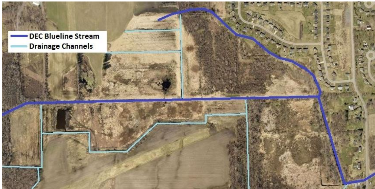
Stream channel has been straightened and drainages ditches are increasing the stream's discharge.
